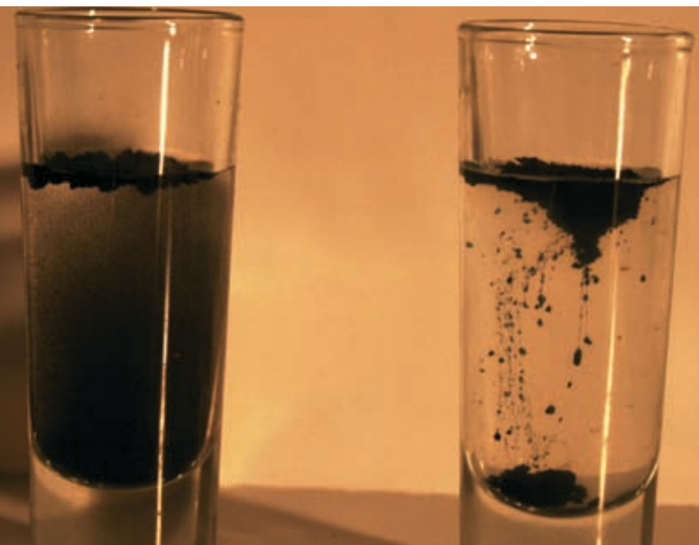
Fine, powdered coal “wetted” with water alone floats on the surface and disperse to completely cloud the glass. Same type dust is “wetted” with water/DC-2008 and fine particles bind together to form larger, heavier particles that sink and never cloud the glass. blending. No dust is generated in this test when treated with AKJ DC-2008.
